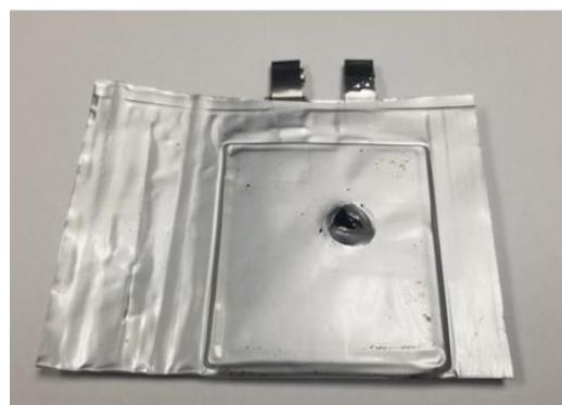
NPORE ® Pouch Cell Survives Nail Penetration Test
